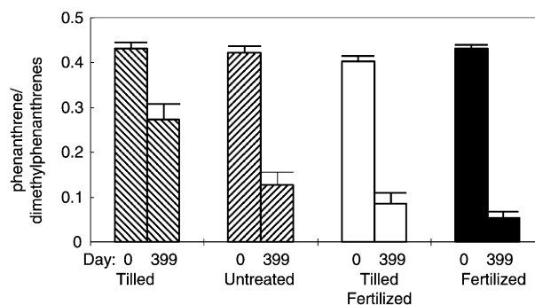
Fig. 9 Changes in the ratio of phenanthrene to the dimethyl- and ethyl-phenanthrenes in oils collected on Days 0 and 399. Error bars reflect the standard error of the estimates. The samples collected on Day 0 on the different plots are statistically indistinguishable, but the differences between Day 0 and 399 are statistically significant ( p < 0.05 ) on each plot.
